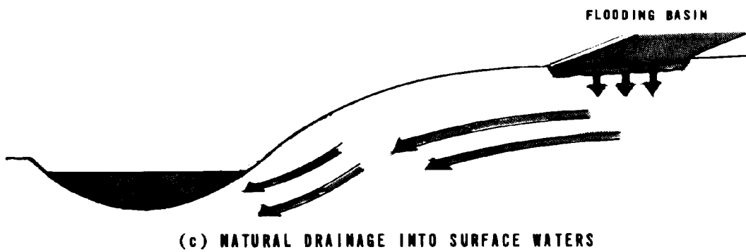
FIGURE 1-2 RAPID INFILTRATION HYDRAULIC PATHWAYS
